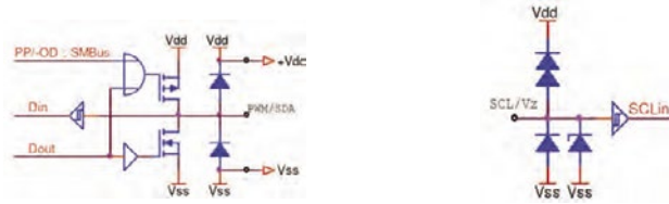
Figure.12 Input / Output pin schematics of TSM
