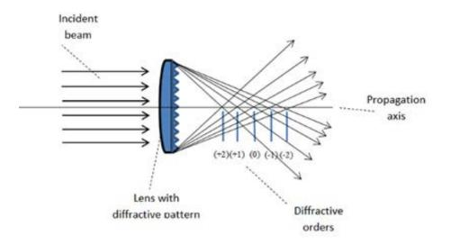
The other configuration is a multi-focal DOE that consists of a window which specified to the case the customer wishes to get a foci spots at a certain distance. This is easily achieved by the addition of a simple focusing lens after the DOE, whose BFL (back focal length) determines the working distance (WD). See figure 2 below.
