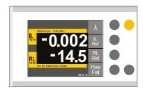
From the measurement screen, press the Pass/Fail Button to display live test results based on the user-configurable settings.
