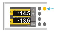
**Note:** It is important that the Return Loss reference is performed where the device-under-test, or DUT will be connected. If a receive cable is being used during measurement, it should not be included in the RL reference.
