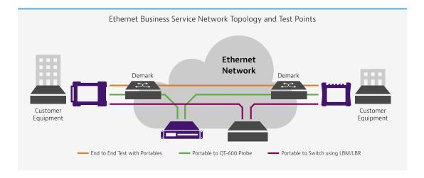
In the diagram above, the "local" TBERD is represented on the left side and the "remote" TBERD is on the right side. The most common service activation use case is a loop-back of the remote device. In this case, the remote device will be the handheld TBERD/MTS device.
