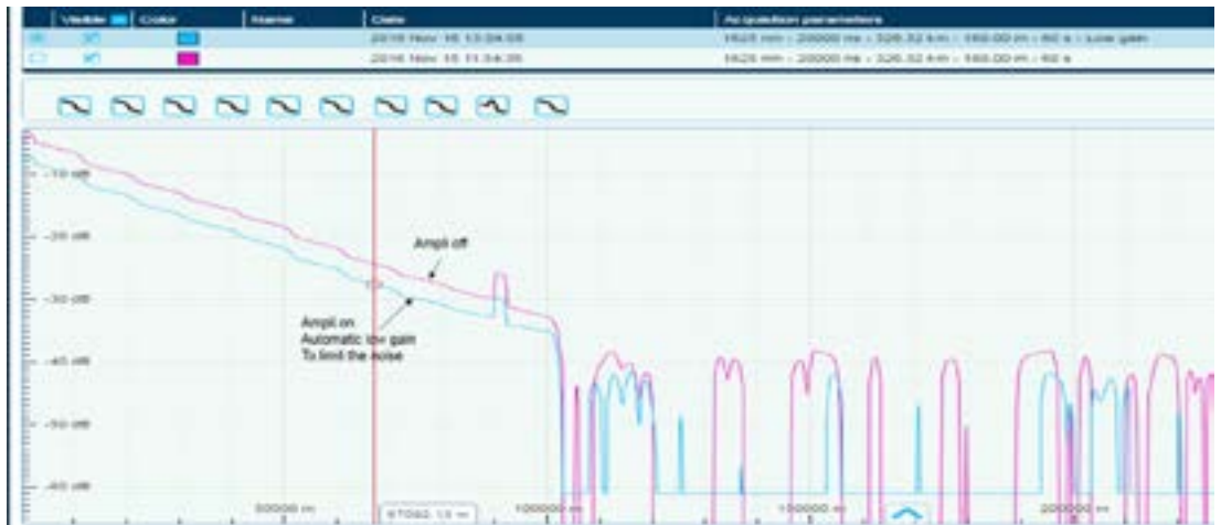
Figure 7: OTDR trace of contra-propagation with Raman amplifier
