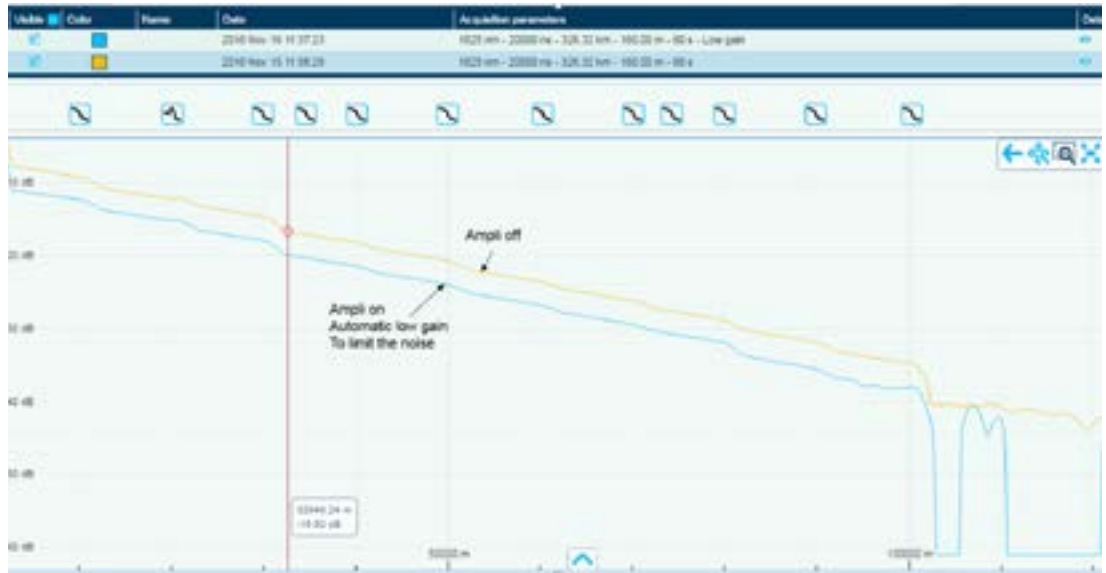
Figure 5: OTDR trace for co propagation with Raman amplifier
