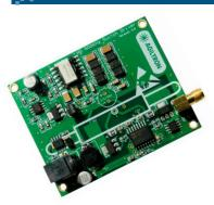
The NSDR series of drivers provide high voltage of signals to drive the NS and NP as well as NF series of solid state switches. The push-pull output design ensures fast transition for both rising and falling edges with the high repeat rate, and it is especially suitable for driving capacitive switch loads.
