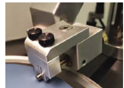
Polishes from 5° to 85° to fiber axis.
