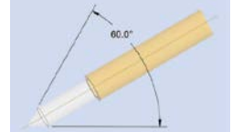
Polishes from 5° to 83° to fiber axis. INCLUDED ANGLES from 10° to 166°
