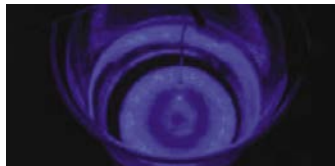
LASER RING BEAM – 351nm laser ring beam is emitted from a 100um diameter optical fiber terminated with a conical surface ground at an included angle of 18.4 degrees. After Watson et al. Dept of Neurology, University of Miami.
