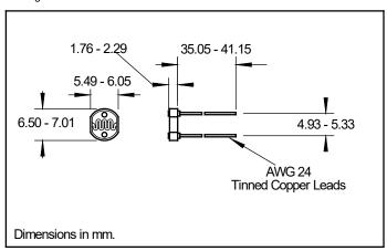
> Soldering Conditions: 260°C 1/16 inch away from case for 3 seconds max.
