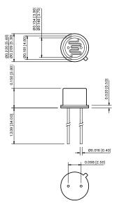
Note: Lead soldering temperature (0.05" inches away from body) 260°C for 10 sec.
