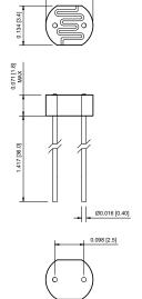
Note: Lead soldering temperature (1/16 inches away from body) 260°C for 3 sec.
