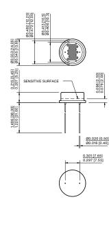
Note: Lead soldering temperature (0.08 inches away from body) 260°C for 5 sec.
