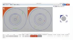
Thanks to its wide field of view camera, the Dscope MT allows to scan both ferrules of Duplex connectors in one shot whether it is LC Duplex or Very Small Form Factor connectors (CS, SN, MDC,...).
