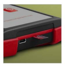
Figure 9: USB interface and microSD card slot
