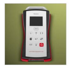
Figure 1: Optical power meter (OPM)
