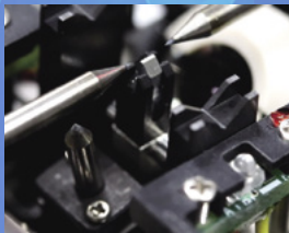
Dual Mirror System-simultaneous view of both fiber ends
