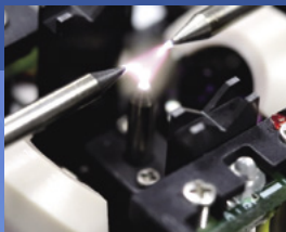
Three electrode Ring of Fire™ arc-discharging and STA²D™
