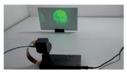
The diffractive approach uning a phase SLM is fairly simple as it only requires a linearly polarized light source and the SLM itself. However, as diffraction angles are limited (dependent on pixel size of the used SLM) it might be necessary to use additional optics to magnify the output image.
