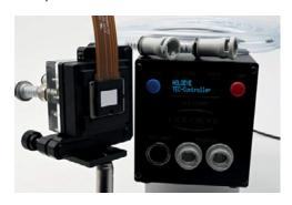
The up-to date display versions of all these SLM platforms use a standardized display packaging with a ceramic stiffener / back plate with excellent thermal conductivity. The displays can be mounted using the integrated magnets or by screws if required.
