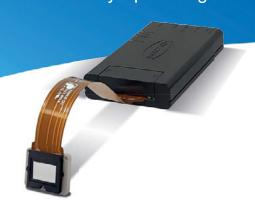
The PLUTO Spatial Light Modulator is the all-rounder within our product range. It is the best qualified and diversified SLM platform with many versions optimized for specific requirements, including high reflectivity versions featuring a dielectric mirror for high power applications.
