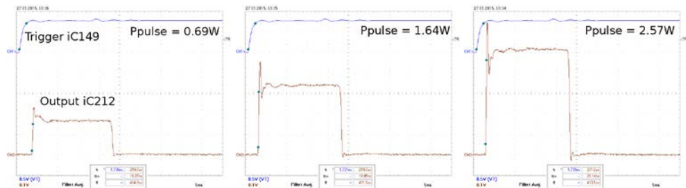
Figure 10: Optical output power at VLDA = 5.5 V, 2 channels. VDD = 5 V, f = 1 MHz, tp = 20 ns
