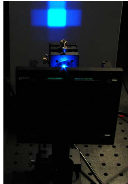
Figure 25: Homogenised blue LED light
