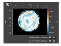
Wavefront error in open-loop WFE = 9 nm RMS
