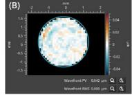
Wavefront error in closed-loop WFE = 6 nm RMS
