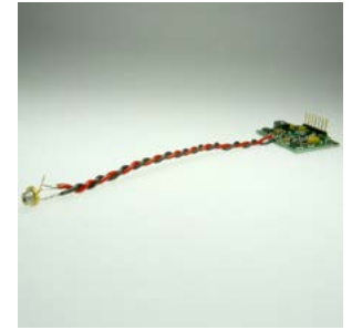
PLD connected by braided wires (length: 100 mm) Current rise time approx. >130 ns
