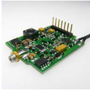
PLD directly connected to the driver Current rise time approx. 3.5 ns
