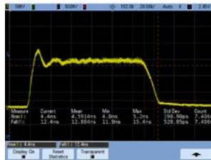
Figure 4: Typical pulse shapes depending on the type of connection between driver and PLD ( V_{op} = 100\text{ V} , I_{op} = 50\text{ A} )
