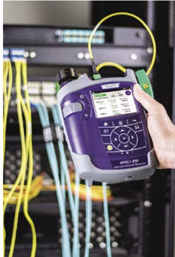
MPOx series OLTS perform Tier 1 certification using MPO connectivity.
