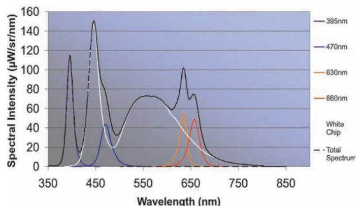
**Figure 7: Spectra of a multi-wavelength LED with five chips and an additional white light LED**
