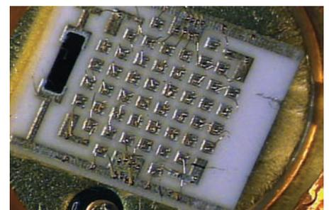
Figure 3: High packing density is a prerequisite for high power LEDs
