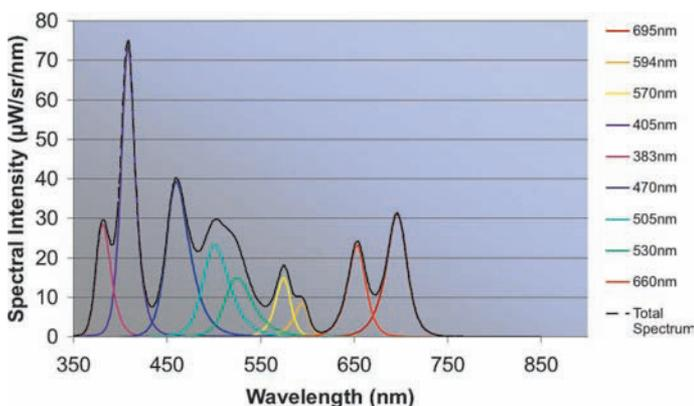
**Figure 6: Individual spectra and complete spectrum of a multi-wavelength LED with nine chips**
