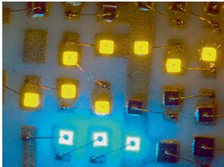
**Figure 4: The individual control of several LEDs with different wavelengths makes it possible to achieve variable emissions spectra**
