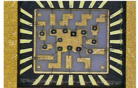
**Figure 5: Lead-free chip carrier for several wavelengths**
