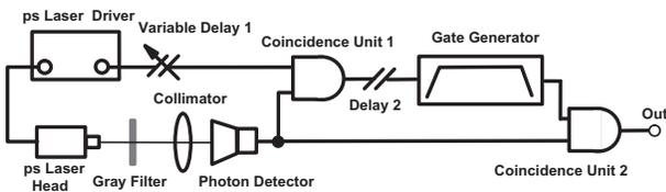
FIG. 6: Setup for measurement of afterpulsing probability.
