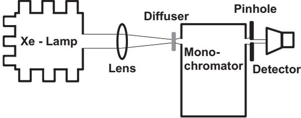
FIG. 14: Setup for measuring relative absolute detection efficiencies at various wavelengths by use of a monochromator.
