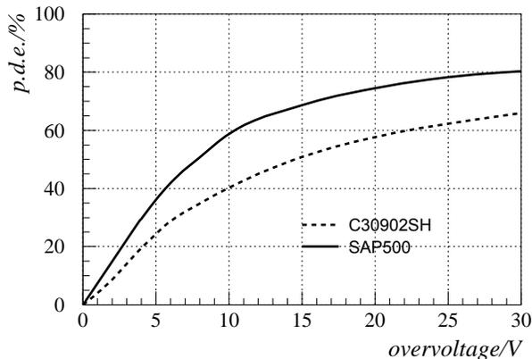
FIG. 17: Photon detection efficiencies as a function of the overvoltage at 676nm. SPADs were kept at  $-23.2^\circ\text{C}$ .
