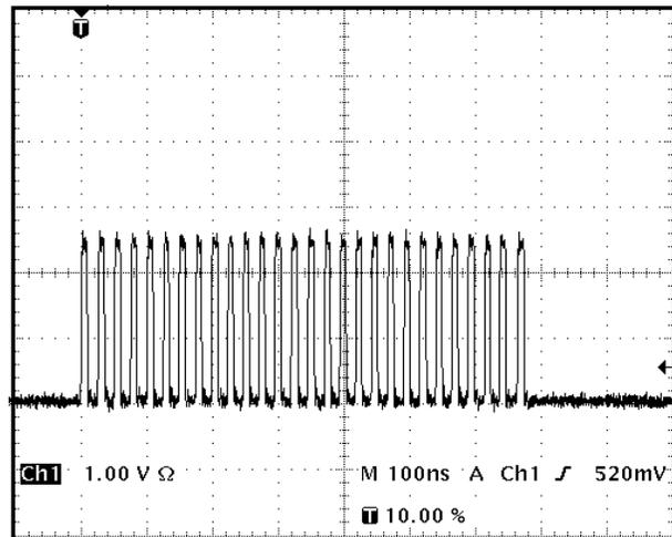
FIG. 9: Inefficient quenching condition at too high an overvoltage - a cascade of quenching attempts.
