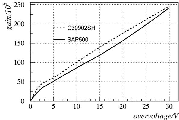
FIG. 3: Multiplicaton gain (in millions) as a function of overvoltage for single photons of 676nm at room temperature.
