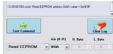
\* Write EEPROM - enable the address field to select address 0-31 of the MD-0003 also enables Value 1 and Value 2 fields for data entry to write at the assigned address.
