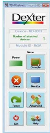
After loading, the software will automatically recognize the TSM type, voltage, SMBus address and open the main screen. The status LED will be GREEN indicating power is applied and communication is established.
