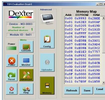
Clicking on the “Memory” button displays the contents of both the MD-0003 RAM and EEPROM in a hexadecimal format. “Refresh” button will re-read the MD-0003, useful with the RAM display to show raw sensor data.
