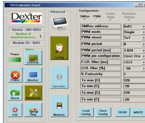
Clicking on the “Config” button allows you to change how the MD-0003 is configured to operate.
