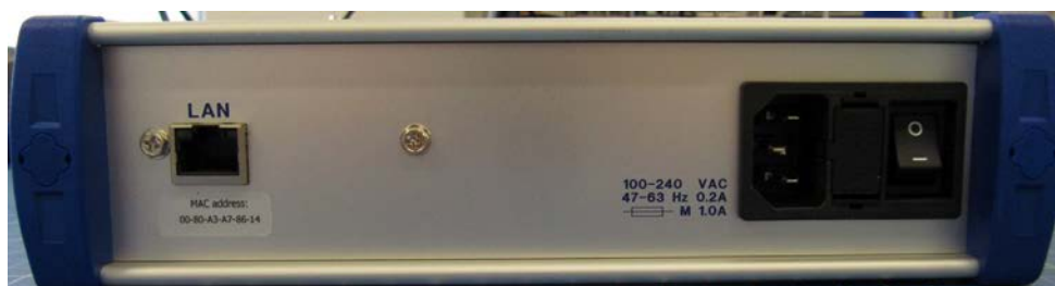
100-240VAC (KG plug) with Ethernet (LAN, RJ-45)
