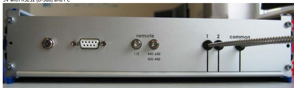
5V with RS232 (D-Sub) and TTL (SMA (remote))
