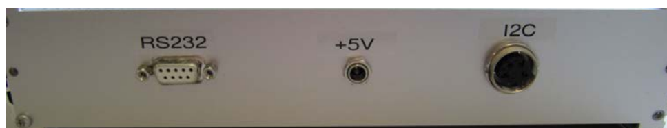
5V with RS232 (D-Sub) and I 2 C
