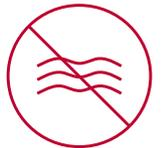
**NEVER** use an ultrasonic cleaner to clean detectors or detector assemblies.
