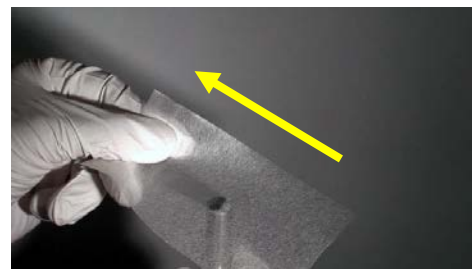
Figure B-3. Wet Tissue Drag across Fiber Ferrule
