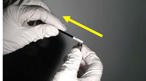
Figure B-4. Swab w/ Methanol - Drag across Fiber Tip
