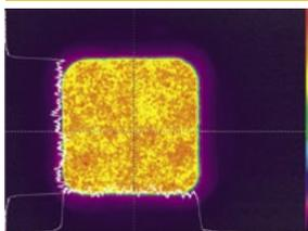
Emitting area: typ. 140µm x 140µm
