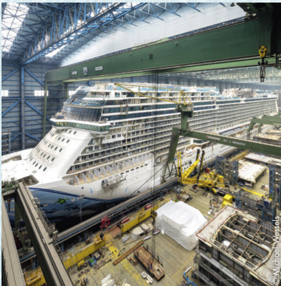
In the construction dock (left), self-levelling lasers (centre) and precision detectors (right) ensure millimetre-precise positioning of the sections weighing several tons.
