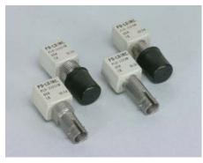
fibre-optic communication solution for 150Mb/s over short and long-range. The sugar cube form-factor allows designers to offer single-mode fibre performance in applications which currently use short wavelength (850nm) components in identical form-factor packages. A link upgrade from multi-mode to single-mode fibre can be achieved by simply replacing the optical components on the circuit board.
