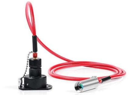
Output coupling collimators: in output coupling, the collimation of divergent light out of the connected fibre is important. The output coupling collimator, which is connected via an SMA connector, is used for this purpose. The optics used are adjustable along the z-axis and are available in three types of coatings from 350nm to 1600nm. To achieve different beam diameters, the output coupling collimators are available in various focal lengths.
