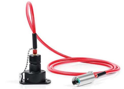
Output coupling collimators: in output coupling, the collimation of divergent light out of the connected fibre is important. The output coupling collimator, which is connected via an SMA connector, is used for this purpose. The optics used are adjustable along the z-axis and are available in three types of coatings from 350nm to 1600nm. To achieve different beam diameters, the output coupling collimators are available in various focal lengths.
