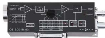
The switchable gain from  $10^2$  to  $10^8$  V/A (decade increments) allows precise and reliable measurements within a very wide dynamic range from nanowatts up to 10 milliwatts optical power.
