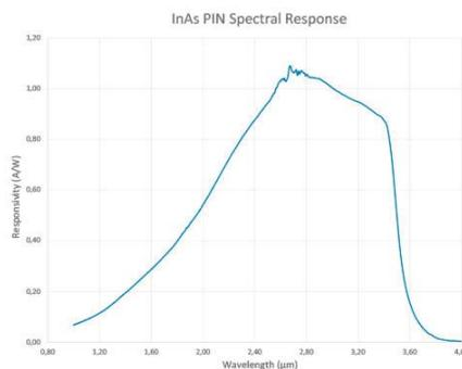
IA35: the IA35 is a heterostructure photodiode on an InAs substrate with a relatively wide peak at  $2.8\mu\text{m}$ . The curve of the spectral response can be seen in the image shown.
