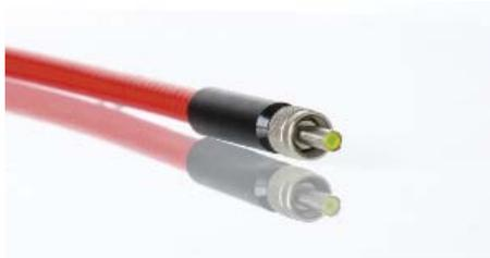
Hollow core fibres use a high reflective coating on the inner surface to confine the light and overcome the high attenuation of silica at long wavelengths. Cleanliness of the inner surface can be maintained by using a ZnSe window in the connector.
