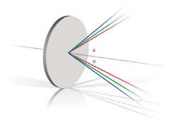
of the wavelengths produced. So-called triple mirrors are used for this purpose, for example in Nd:YAG laser systems that emit at the fundamental wavelength 1064nm and have harmonics at 532nm and 355nm, a
