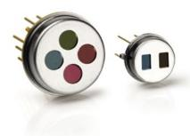
The devices are manufactured in standard TO style packages that can be fitted with a range of windows including CaF<sub>2</sub>, KBr, BaF<sub>2</sub> and ZnSe-Ar. Thermoelectric coolers can also be supplied in TO-99 and TO-37 packages, the TEC can be used to tune the detector temperature to maintain maximum responsivity.
