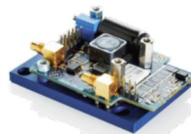
communication with a PC for control of pulse current, pulse duration and repetition rate, or via the external PLB-21 User Control Unit. ■
