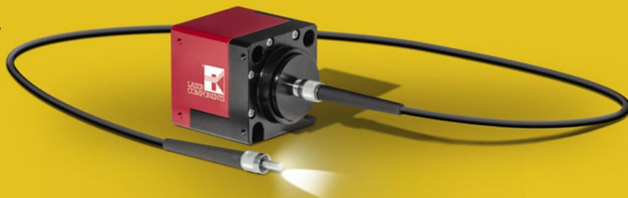
The light source is the innovative laser light technology from SLD Laser. Two semi-polar blue GaN laser diodes (450nm) illuminate a phosphorus chip, producing a brilliant, incoherent white light that is more than ten times brighter than the brightest white LEDs available.
