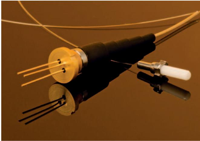
**FAC Lenses.** LASER COMPONENTS Canada offers pulsed laser diodes (PLDs) with integrated microoptics, a so-called fast-axis collimation lens. Mounted directly in front of the laser diode chip, the divergence of the “fast” axis is reduced to 5 or 10 mrad.
