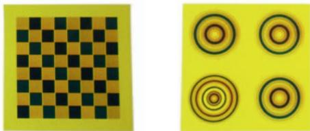
The structures can be designed to feature different optical properties such as orientations of the polarization axis or wavelengths surrounding 600 nm and 800 nm featuring extinction ratios above 1,000 : 1. The polarizers can be supplied in various shapes and sizes.
