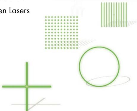
Because the green 520nm wavelength is becoming more and more popular, we have expanded our product range with a number of new DOEs for green light, including a cross hair that has a fan angle of more than 50°, and a DOE with 15 parallel lines. ■
