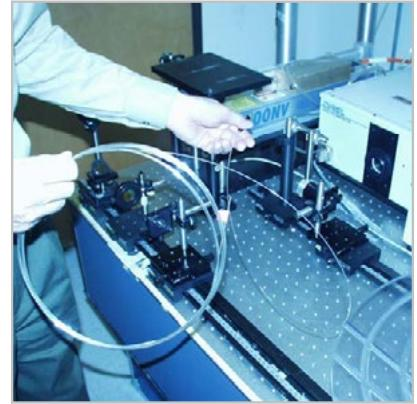
Figure 2: Hollow Silica Waveguide In Use
