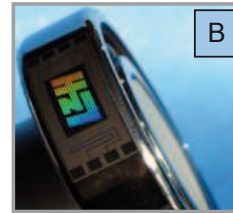
MID on flexible polymer (A) and strain gauge on ball bearing (B)
