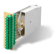
Example for a module assembly: Splitter 3-fold 1x4 in a vertical plug-in module 3 HU with connectorized output fibers and input fibers mounted into a splicing cassette
