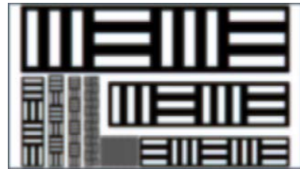
Resolv4K Zoom @ 4.5X High Mag 8.9MP Sensor – 0.76µm / pixel 3.56mm FOV – 5.20mm² Area (3.25X more)
