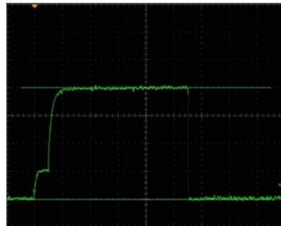
Figure: Output signal for a 50 µs / 50 A prepulse and 200 A / 500 µs main pulse
