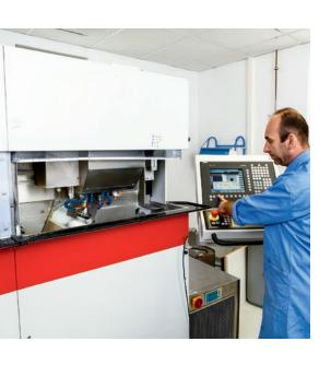
In order for us to offer quick service, we manufacture laser optics substrates directly in Germany – from single items to small series. You determine the material used in your laser optics: Different fused silica glasses are recommended for high laser power, and the inexpensive N-BK7 is recommended for low power.
