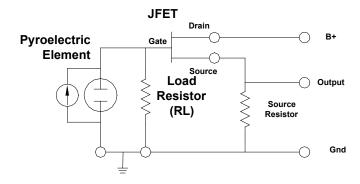
The input load resistor RL is a major contributor of noise as it produces Johnson noise (VnR) which is defined as:
