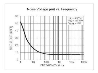
The graph above shows the *en* voltage noise as a function of frequency of a JFET which would be used in a detector for a high frequency application. Note the *en* at 1.0 kHz is about 6 nV
