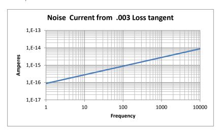
Note the change of the loss tangent noise with frequency. As the frequency increases the noise increases as the square root of the frequency. This shows that the loss tangent noise is more important at higher frequencies.
