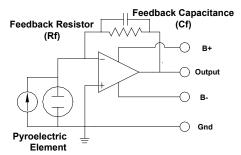
The higher output comes about by the fact that in the CM the Opamp's feedback loop impedance is much greater than that of the VM. The only capacitance in this loop is the very minimal stray capacitance (~0.2 pF) where in the VM the capacitance could be 10 to 100 times larger.
