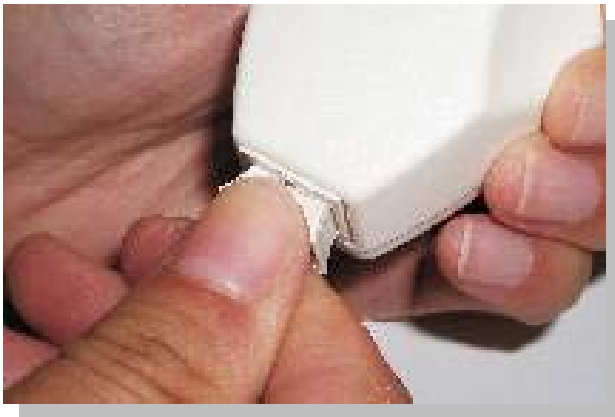
FIGURE 3 Insert POF into OptoLock.
