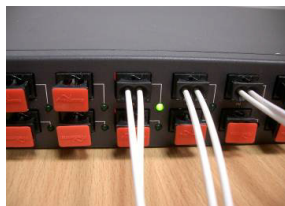
FIGURE 8 If the link is fully connected the indicator LED will flash showing activity on the Ethernet link.
