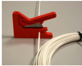
FIGURE 1 Slice the POF cable.
