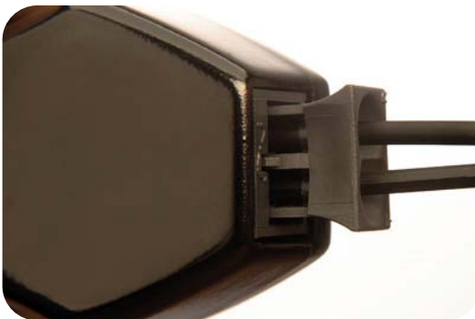
Figure 3. Insert POF into OptoLock.
