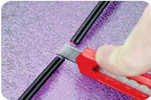
Figure 1. Slice the POF cable.
