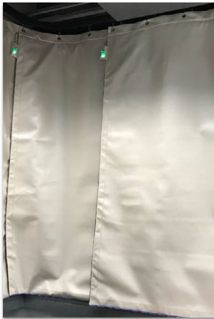
Active laser protection curtains connected in series
