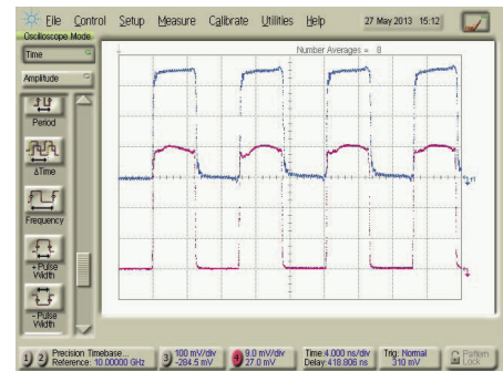
Electrical pulse from AWG (blue curve) with corresponding Optical output (pink curve)
