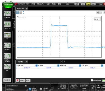
Input signal: Pulse amplitude = 0.25 V pp , Rise time = 32 ps
